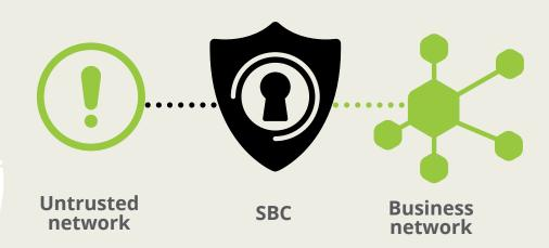
An SBC resides on the border of the network connecting directly to all SIP peers - This will usually have a direct interface on your WAN or DMZ network. The application layer will reside behind the SBC and will connect to the SBC's LAN interface. This segrigates traffic not only logically, but physically as well.
